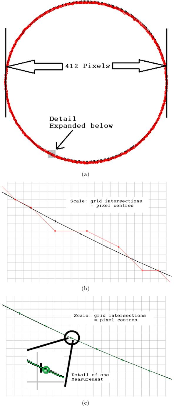
**Fig. 7** (a) Evaluation data shows circular plot recorded. (b) Point photo detector and ideal line shown with zoom at pixel level. (c) Planar photo detector and ideal line shown with zoom at pixel level.
