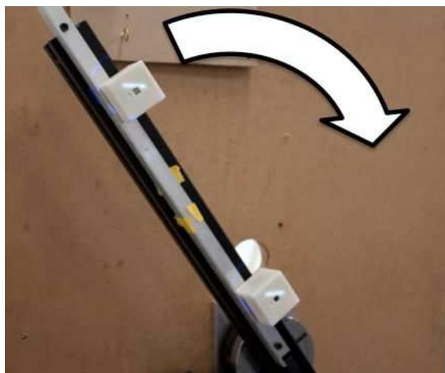
**Fig. 5** Computer controlled rotating arm for precise movement.
