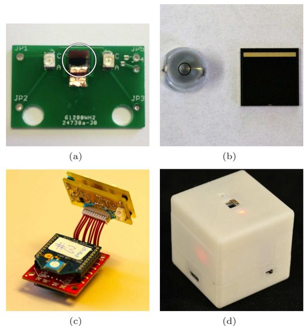
**Fig. 3** Hardware Components. (a) Close up view of planar photo detector shown in white circle. (b) left - Top view of point size detector with lens, sensing element is shown with black circle. right - Planar photo detector. (c) Electronic components including Arduino Pro Mini, Xbee wireless, amplified planar photo detector. (d) Generic photo detector node in 3D printed case.
